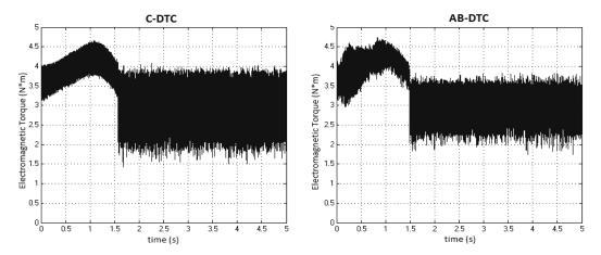
Figure 6. Electromagnetic torque responses at loaded working conditions
