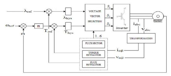
Figure 2. The block diagram of the conventional DTC
