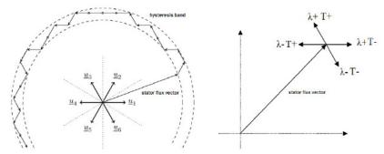
Figure 1. The rotation of the stator flux vector and an example for the effects of the applied inverter switching vectors [16].
