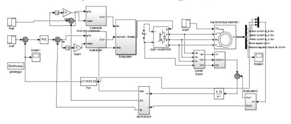
Figure 4. The proposed AB-DTC system with the Simulink blocks
