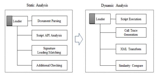
Figure 3. Configuration of Web Content Analytics Engine
