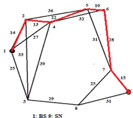
Fig.4 Optimal Path using traditional ACO
