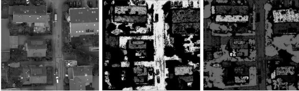
Figure 5. Base image (left), Segmentation of surface normals in object space using second algorithm (middle) and image space (right),  $\theta < 11.5^\circ$ ,  $r < 0.4$  m, 250 nearest neighbors, nDSM threshold = 1.5 [m]
