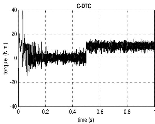
Figure 9. C-DTC torque response
