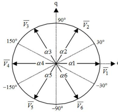
Figure 1. Inverter voltage vectors and sectors
