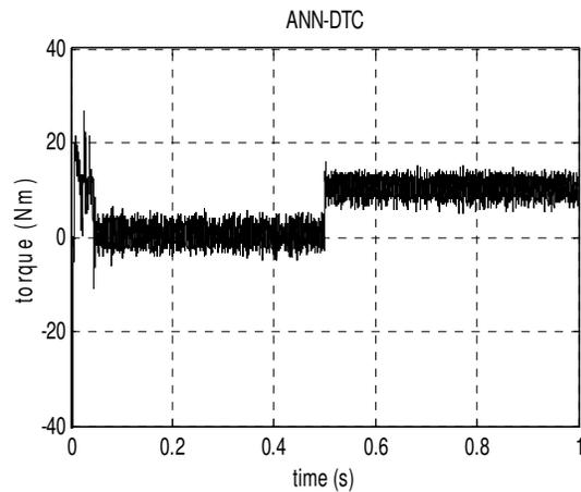
Figure 10. ANN-DTC torque response
