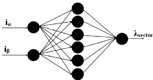
Figure 2. Stator flux sector determining ANN structure
