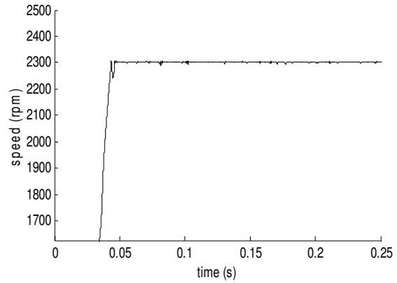
Figure 8. ANN-DTC speed response at startup
