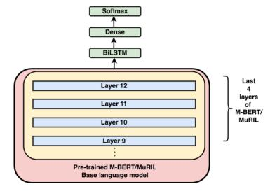
Figure 2. M-BERT/MuRIL-Bilstm architecture
