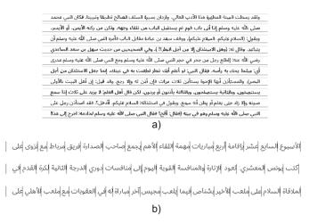
Figure 2. Examples from Preprocessing Stages: a) cut indices for line segmentation, on document b) cut indices for word segmentation, on lines
